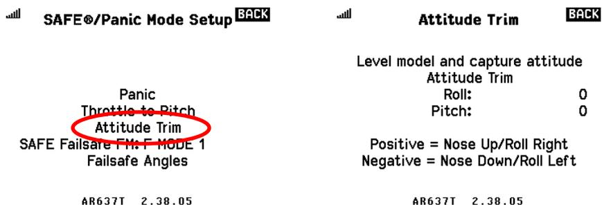
As with the First Time SAFE Setup, you can either set the plane in a level flying attitude (prop up the tail on a tail-dragger) and let it suggest settings for the trim by selecting "Level model and capture attitude", or you can adjust the trim manually.
