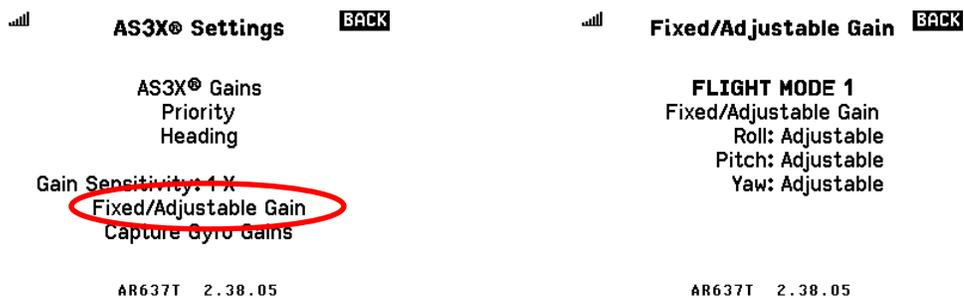
For each flight mode (don't forget to flip the flight mode switch to see them all), set each axis to either Fixed or Adjustable.
