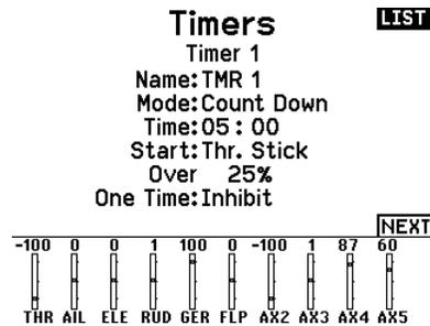
Change the time to a value that's appropriate for your model and flying habits. If you're not sure which value to use, consult the manual for your model. Note that it is not good for the batteries to keep flying until the motor reaches the Low Voltage Cutoff warning. You want to land before that happens! Over time you'll find the optimum setting for the timer based on your flying habits.
