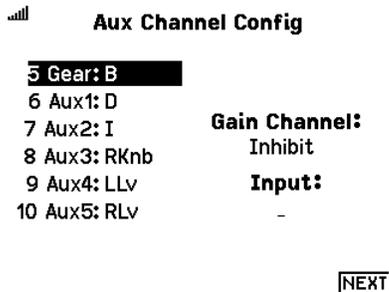
You must assign a channel for that purpose here (as shown). There will be more on how to use this feature later, but for now I’m going to go ahead and assign Aux3 (the knob) to “Gain Channel”.
