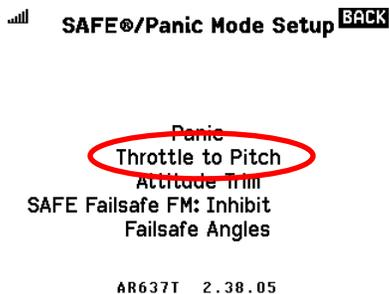
This mix has two parts – a low end and a high end. On the low end, if the throttle is below the threshold percentage, then input will be applied to the pitch. Similarly, on the high end, the input is applied when the throttle is above the threshold percentage. The input applied is linear, meaning that it applies partial elevator input proportional to the amount of throttle applied, increasing with the maximum elevator input applied at either 0% throttle (low end) or 100% throttle (high end).
