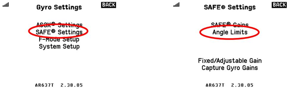
That will take you a screen where you can adjust the angle limits for each flight mode by flipping the flight mode switch.
