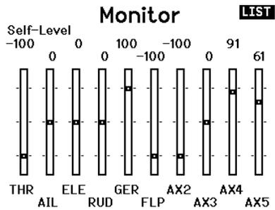
The AIL, ELE, and RUD channels will move with the sticks. Go ahead and play with it. **BE CAREFUL WITH THE THROTTLE IF THE PROPELLER IS MOUNTED ON THE PLANE!**
