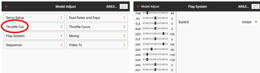
Change the Switch setting from “Inhibit” to the switch you want to use for the flaps. This is where you set the flap control for each switch position, along with any additional elevator input, and the speed at which the flaps move. The Flap System will automatically associate the switch with the Aux1 channel.
