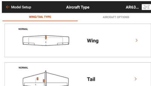
By default, the wing and tail type are both “Normal”. For a plane with simple controls for elevator, aileron, and rudder, leave the Wing and Tail set to Normal.
