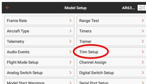
Change aileron, elevator, and rudder from “Common” (same settings all the time) to “F Mode” (different setting for each transmitter flight mode).
