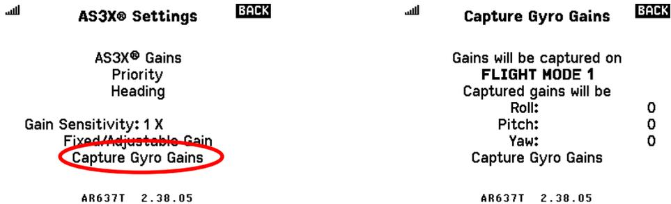
Not only can you see the gains here, but you can capture or save the current levels as the new gain settings for the current flight mode. When you select “Capture Gyro Gains”, the receiver will save the current adjustable gain values as the permanent values and change them from being adjustable to being fixed.
