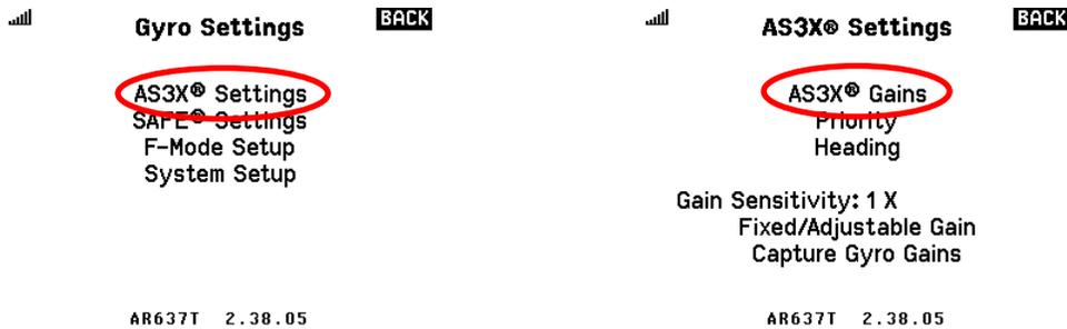
Select "AS3X Gains" on the AS3X Settings screen, and then you'll be able to set the baseline rate gains for each flight mode. **As with similar screens with a choice of flight mode, flip the flight mode switch to change which mode is being adjusted.**
