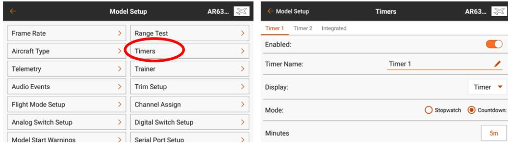
Change the time to a value that's appropriate for your model and flying habits. If you're not sure which value to use, consult the manual for your model. Note that it is not good for the batteries to keep flying until the motor reaches the Low Voltage Cutoff warning. You want to land before that happens! Over time you'll find the optimum setting for the timer based on your flying habits.
