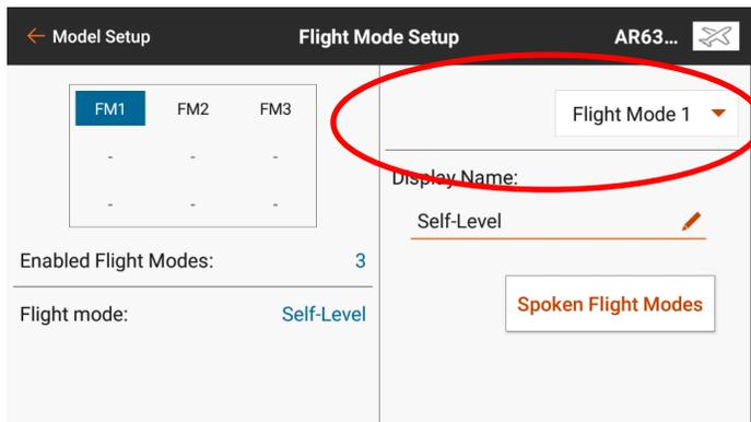
Flip switch B to change the current flight mode, and touch the Display Name to change the name of the other two modes.
