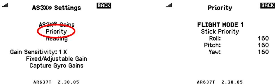
The Priority setting controls the balance between stick input and automatic reaction from AS3X. The default setting is 160% for all axes, and that seems to be a good starting point for most models.
