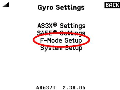
This is where you set additional features that will be active in each flight mode. As usual, use your flight mode switch to change the screen from Flight Mode 1 to Flight Mode 2 to Flight Mode 3.
