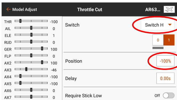
When you use Forward Programming to configure the receiver and Throttle Cut has been set up, then you must turn on Throttle Cut to get into the Forward Programming menu. This is a safety feature.
