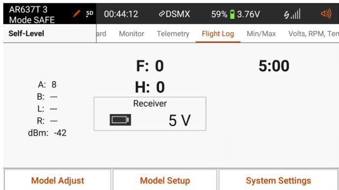
After you bind the transmitter to the receiver, go to the Model Setup menu and choose Telemetry. You can see all of the sensors the transmitter has detected while binding.
