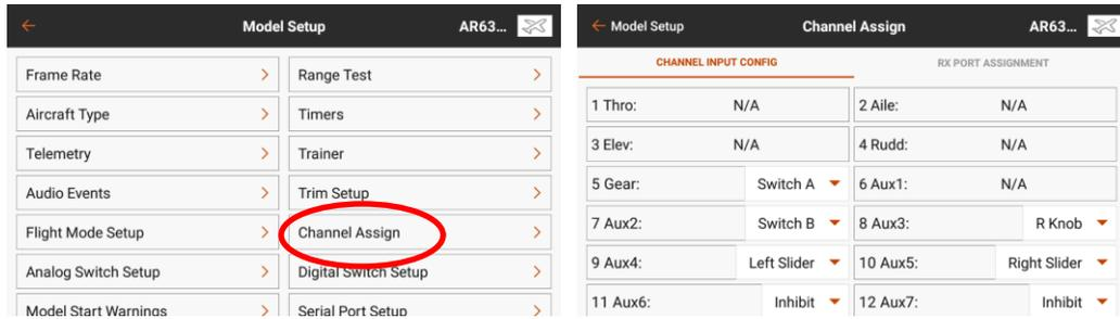
On the Channel Input Config screen, you map switches to radio channels. Make these changes:
