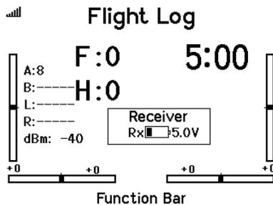
After you bind the transmitter to the receiver, go to the Function List menu and choose Telemetry. You can see all of the sensors the transmitter has detected while binding.
