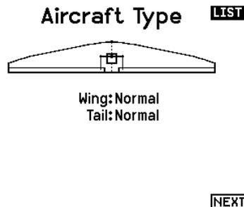
For a plane with simple controls for elevator, aileron, and rudder, leave the Wing and Tail set to Normal.
