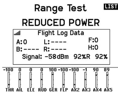
You’ll see the signal strength level at the bottom in both dBm (the technical measurement) and a percentage. The dBm reading should be somewhere between -40 dBm (about as good as it gets) and -85 dBm. Anything worse than -85 dBm would be considered poor reception.
