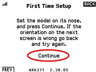
After that, the receiver will display what it believes is the detected orientation. (If you instead choose to set the orientation manually, you get to this screen directly.)
