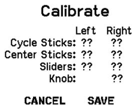
On this screen, move the sticks slowly in the shape of PLUS SIGNS, not circles. Move each stick up and down, back to center, and then left to right. Do not push hard to move the stick to the edge of its movement. Repeat the movement a couple of times until the screen shows “OK”
