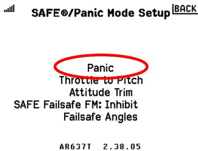
The settings in Section 2 assigned the panic control channel to be Aux 2. I also adjusted the envelope limits to be a lot tighter, especially for pitch (nose) down. You also need to select a flight mode that Panic should use for gain settings. Select the flight mode that has self-level enabled.
