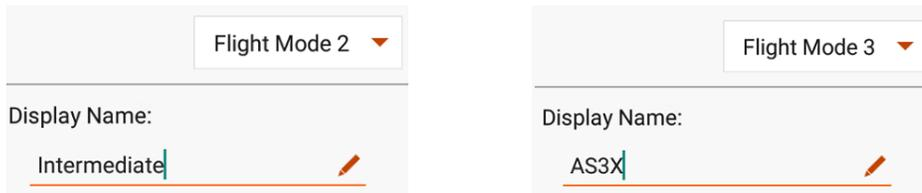
By default, the iX will speak the Display Name for each flight mode. If you need to adjust the spoken version of the names, touch the “Spoken Flight Modes” button.
