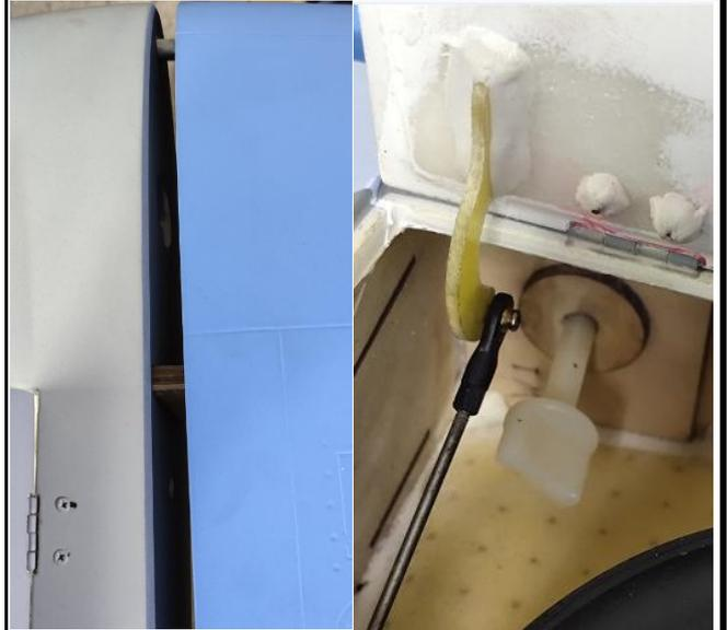
11. Assemble the wing to the fuselage and lock it with screws.
