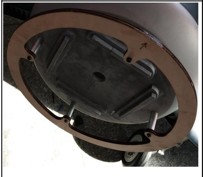
19. Install the engine to the firewall with screws, put the cowling to the engine and glue the cowl to the ply wood frame.
