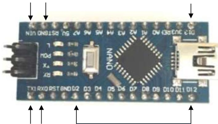
Power to the Arduino is provided at the VIN (+5V) and GND pins (marked by arrows in the pinout). These can come from the receiver SRXL2 connector too. The PWM signal outputs come from pins D2 through D13 and will drive servos directly (D13 is on the opposite side of the board from the other outputs). D2 is the throttle channel, D3 is aileron, D4 is elevator, etc. D8 will be AUX2, D9 = AUX3, etc.
