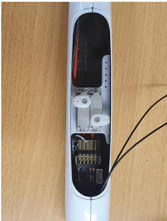
At this stage, building was looking great and I went for the steel cable guide tubes (supplied). Tube was cut in half which means it could guide the cables past the wing. I took
