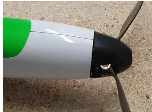
From the inside add 2 drops of medium CA and rotate the fuselage until the firewall has glues all around (that's why I liked the sealing), finally add filler (speedy pulver). Epoxi would be fine too.
