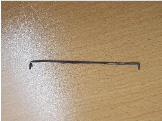
Install the rod entering from the top skin slit, attach to servo and horn. Make sure servo is centred, servo arm is offset towards the leading edge and glue the horn, as you see the pushrod has to move lower than the top skin for full flap deflection.
