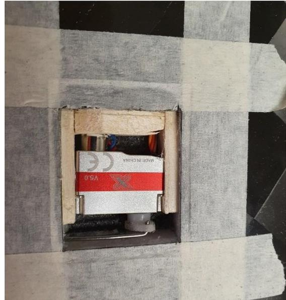
Balsa is glued with CA to the wing while servo receives a couple of epoxy drops. Since they are metal casing it is easy to remove with some heat. Don't forget to cut the servo plugs and push the wires towards the centre of the wing (channels are factory cut in the core).
