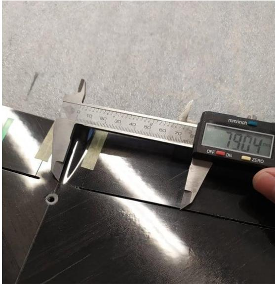
Mark the horn position, offset sideways from the rod.
