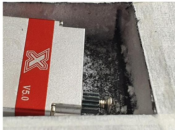
With help of light reflection you can see where it would exit in the top skin trailing edge, mark that position. Mark a position 15mm in front of it and drill the skin.
