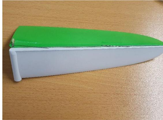
Insert the rudder and bolted the elevator to their places. With a pen, mark where the control horns should be (special attention in the elevator as clearances are small).
