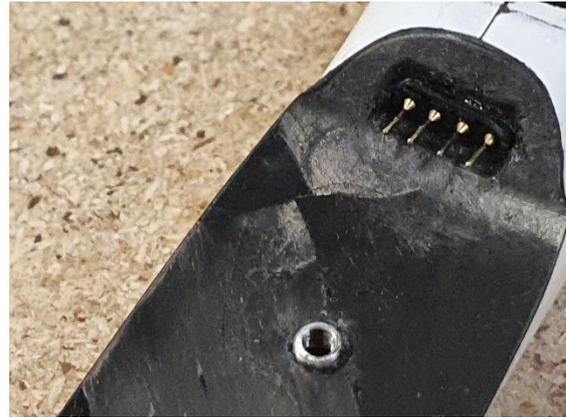
In case you, like me, forget where positive and negative are know that there is no continuity between positive and signal but there is a high Ohmic, continuity, 1.6k between signal and negative, at least in KST 08 servos
