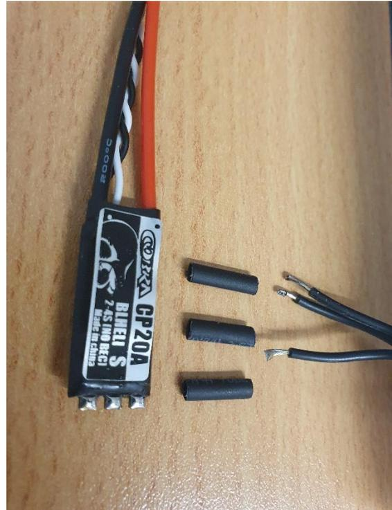
As you can note, drone ESCs do not have BEC so they do not have the red wire going to the RX. The reason I liked the suggested power train is that it operates very well in 2S. Hence, I installed the red wire, soldered to the battery wire terminal of the ESC and added the pin to the RX connector. This means RX and servos get battery voltage directly from the source, so it only works with 2S!
