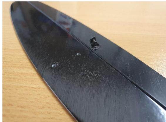
Foam is removed and horn glued in position with Epoxi. As you can see, I accidentally used one the aileron horn in the rudder, no big deal.
