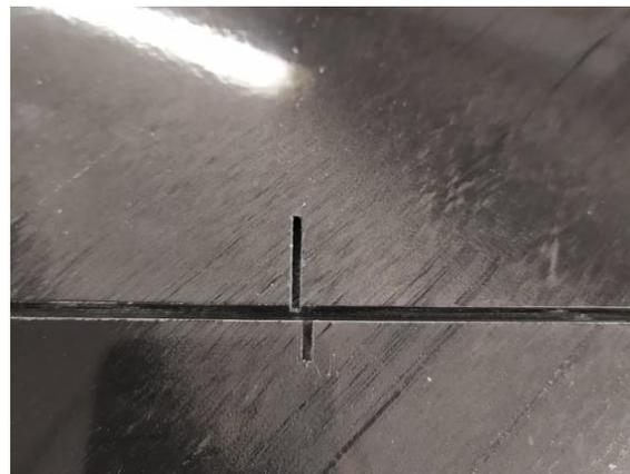
Prepare your servos by centring them and cutting the servo arm to the first hole. When inserting the servo arm to the servo make sure to offset it from center position, this way you have more throw capacity to deflect the aileron/flaps down than up. Bend the push rod 90 degrees attach it to the servo arm and install in the wing channel. Insert the horn and mark where the push rod has to be bent,
