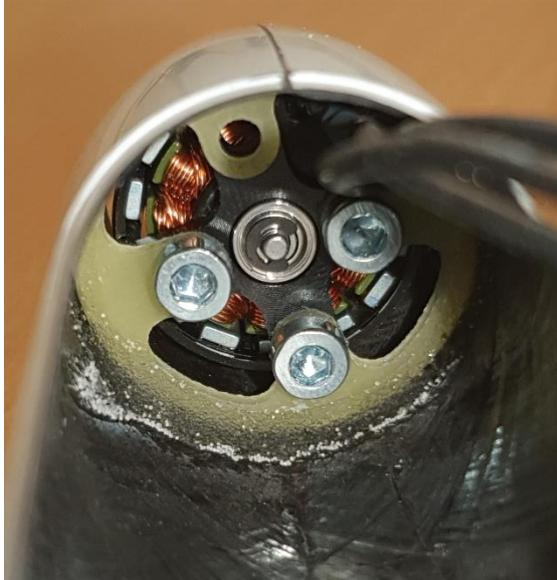
Note the motor final position in relation to the fuselage edge.
