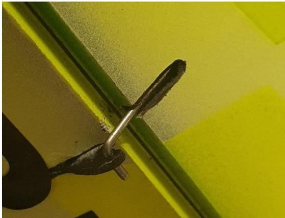
I used Oleg's suggestion of servo mounting by filling the spaces in the servo pocket with light balsa.
