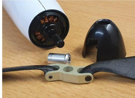
Push the motor again and voila! No friction and very small gap.
