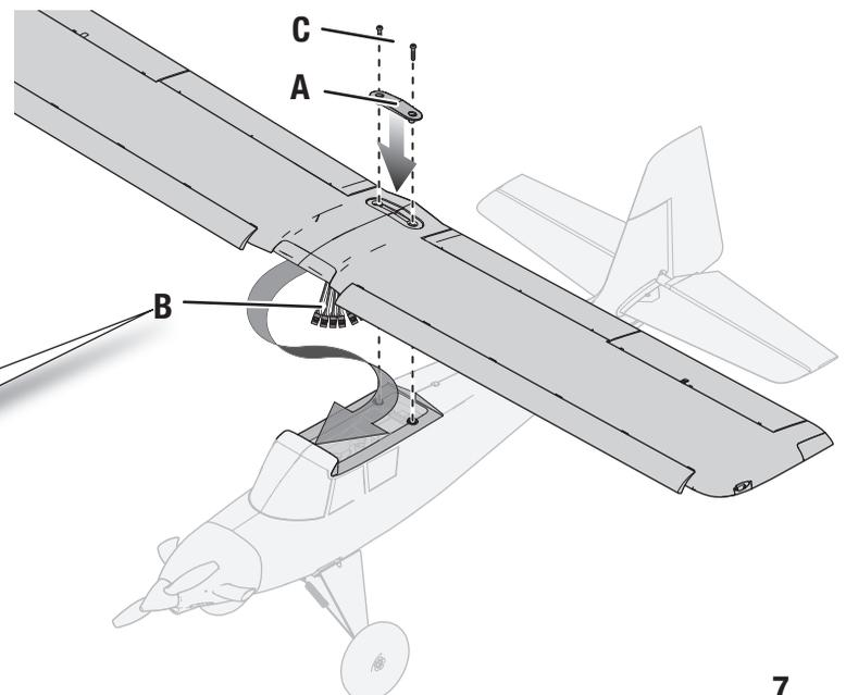
**CAUTION:** DO NOT crush or otherwise damage the wiring when attaching the wing to the fuselage.
