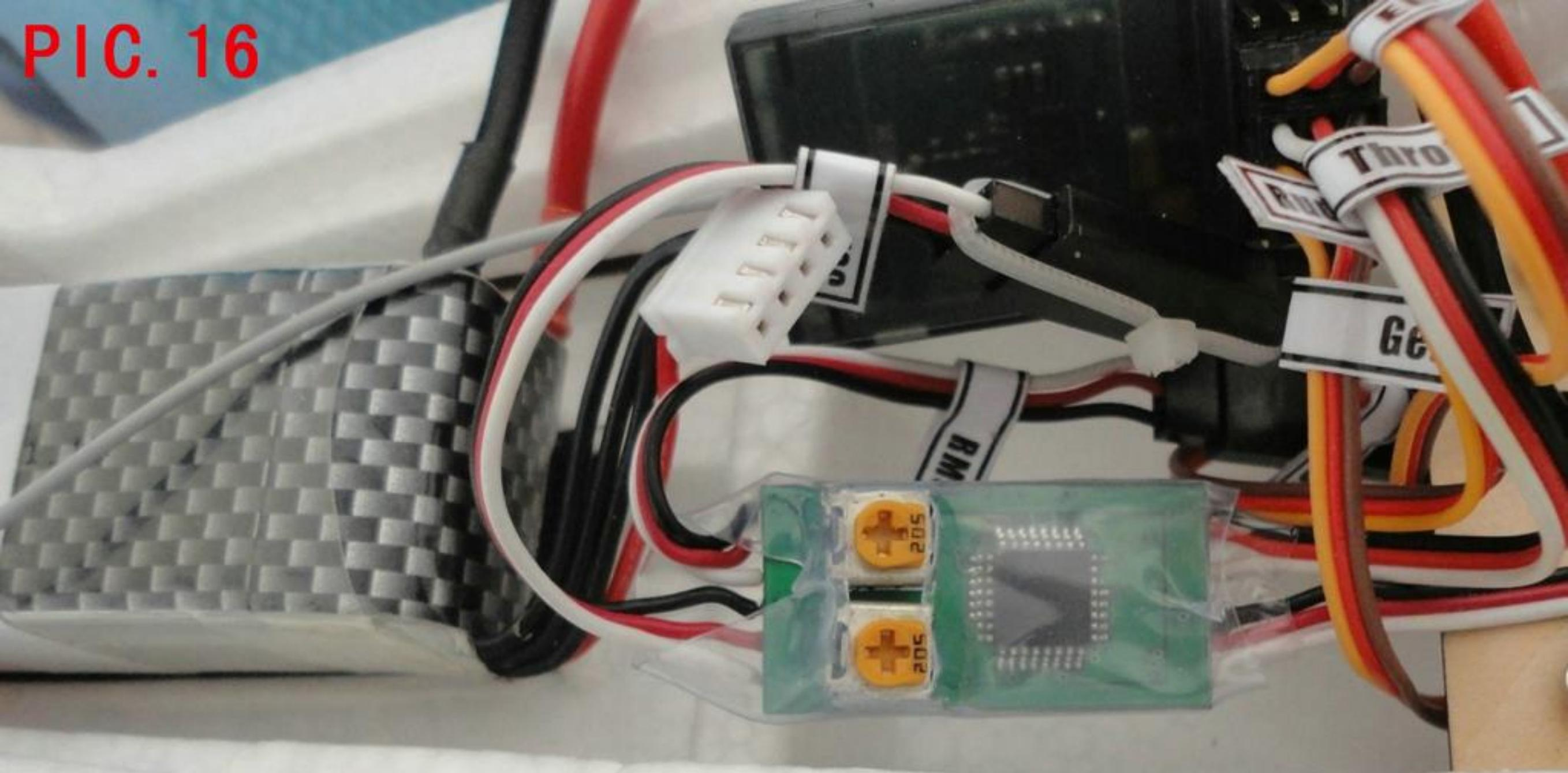
Set the low end point adjusters of RMS servo in their mid position
