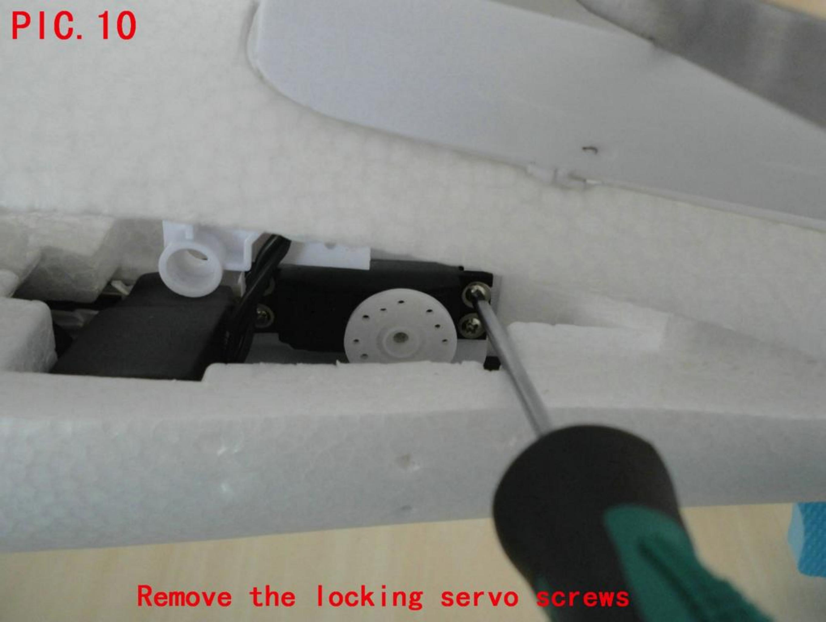
**Remove the locking servo screws**
