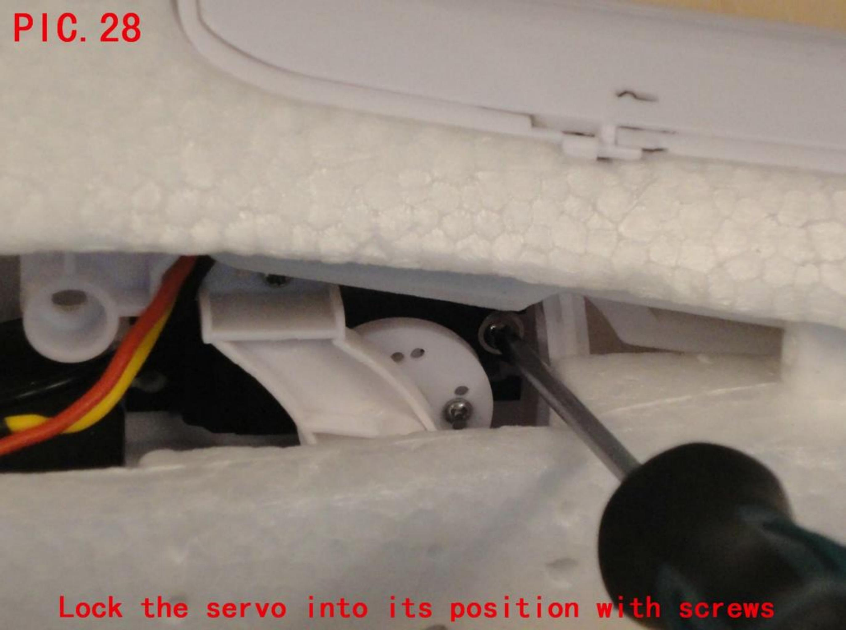
**Lock the servo into its position with screws**
