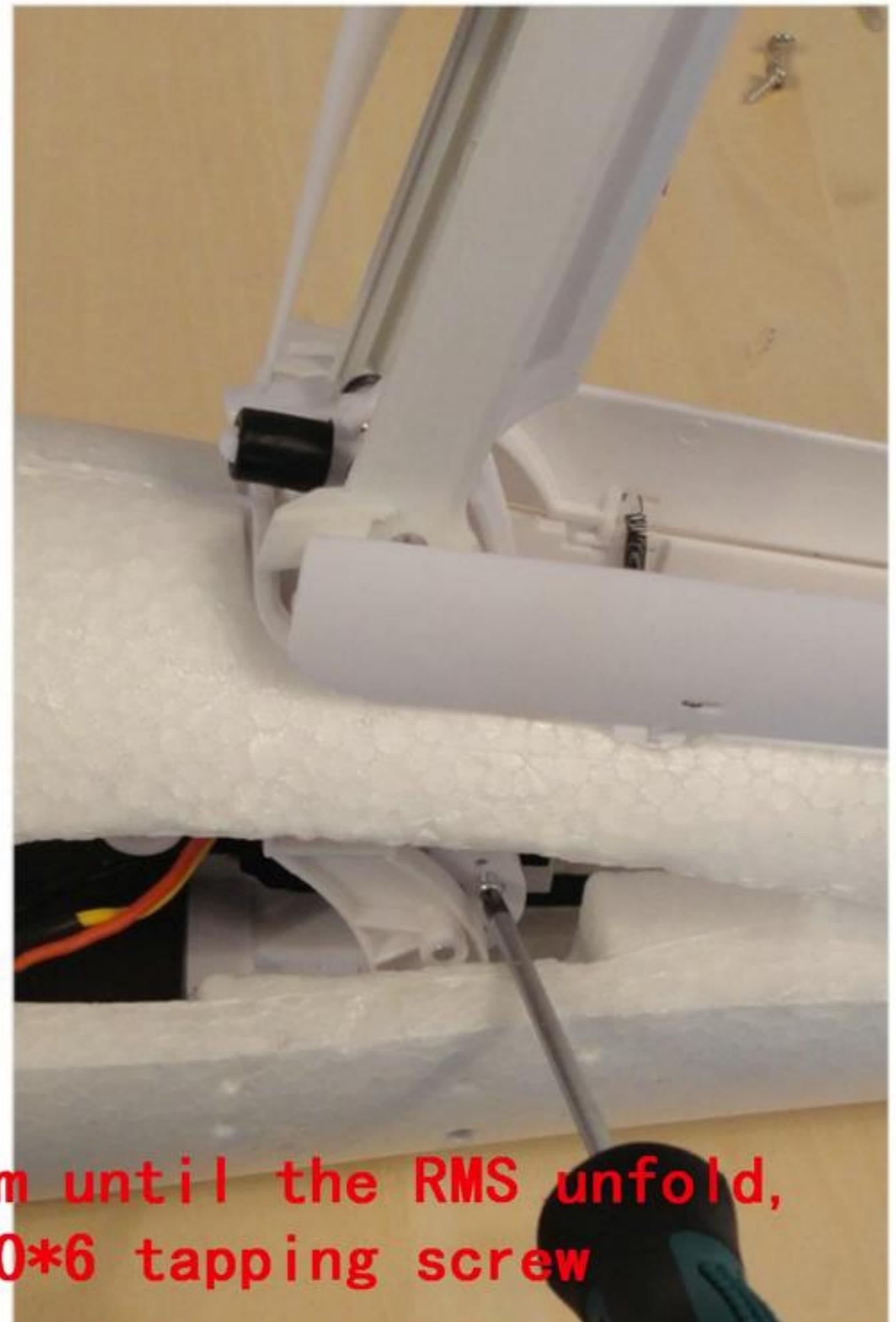
Upward the throttle trim until the RMS unfold, then lock the other M2.0\*6 tapping screw
