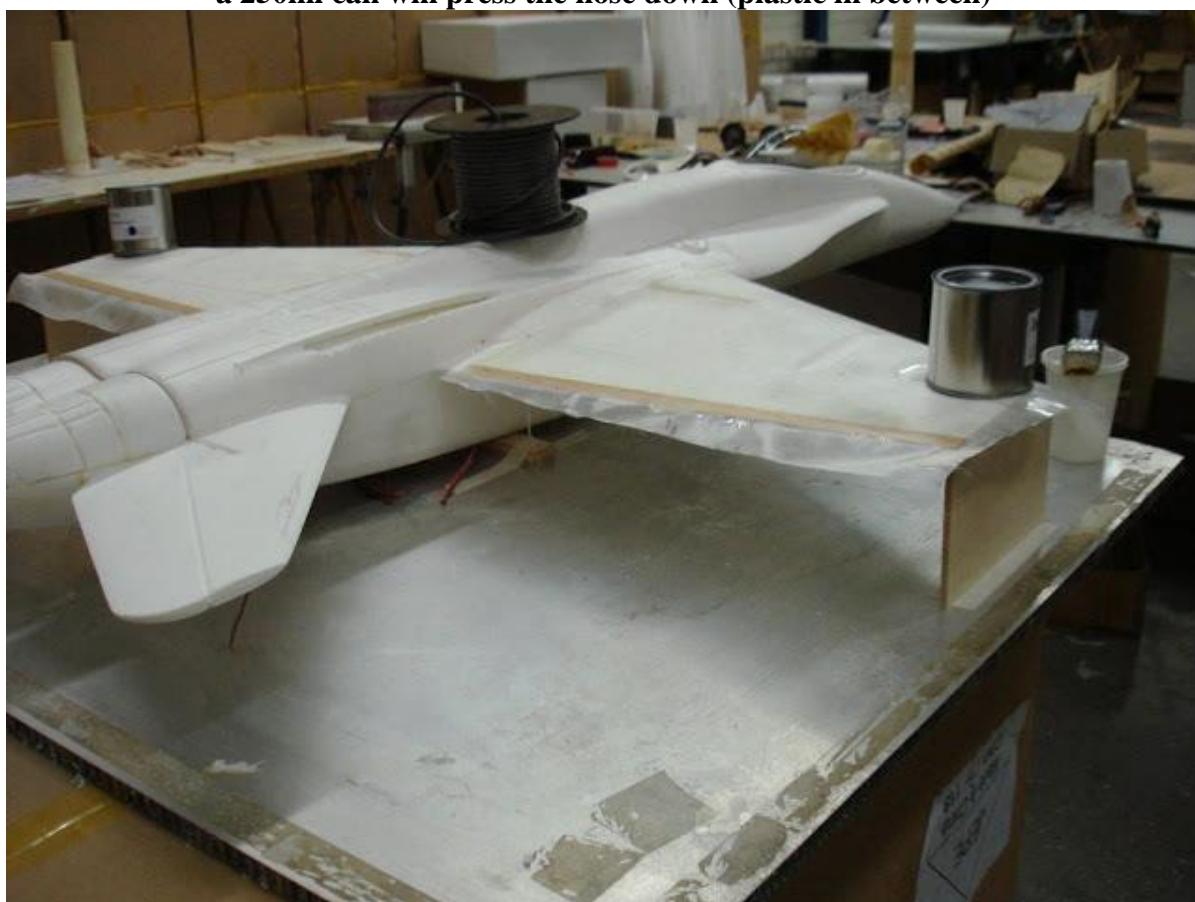
tissue is not cut on trailing edge (only finished at leading edge)
