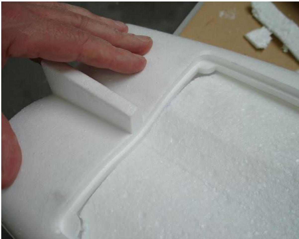
test good fit of bottom half of fuselage (do not glue yet)
