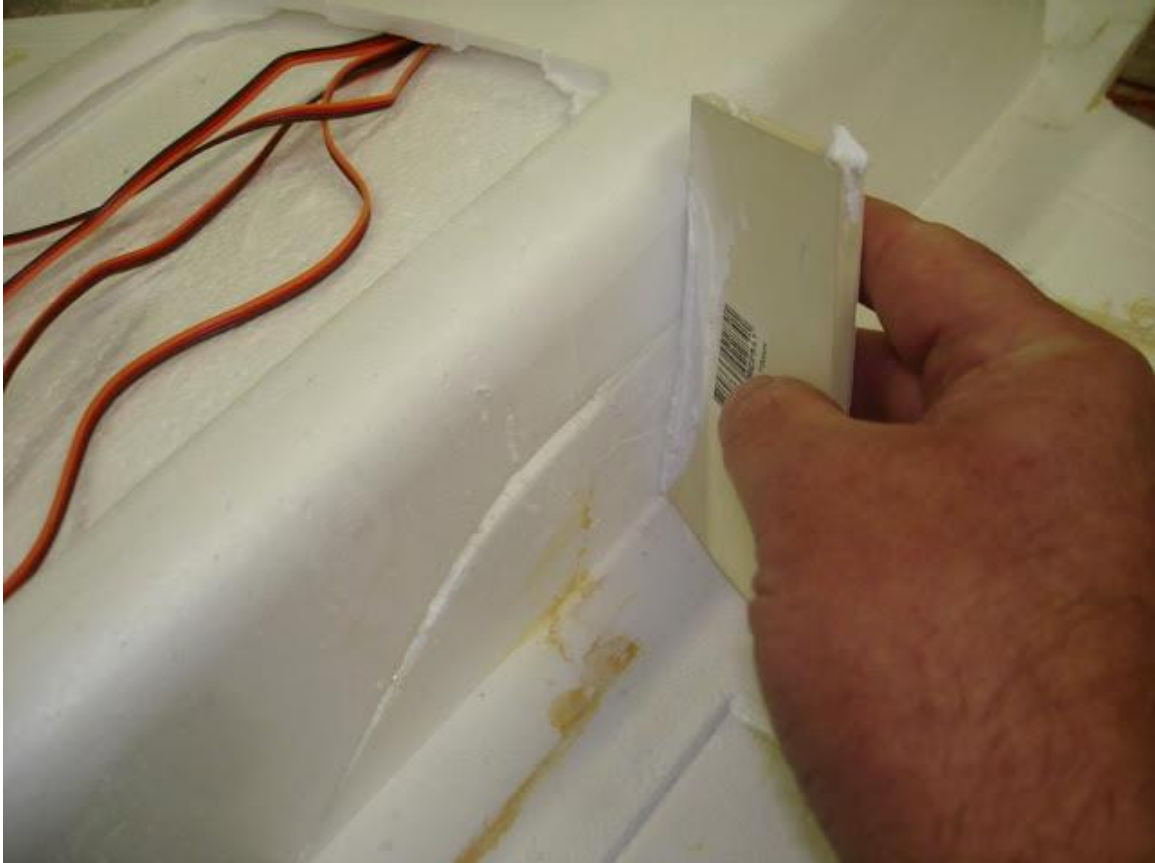
clean up the fuselage join with Easy Filler
