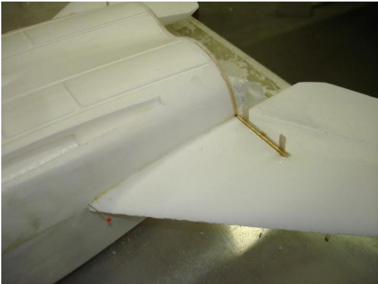
glue elevator to fuselage and bulkhead with some PU glue
