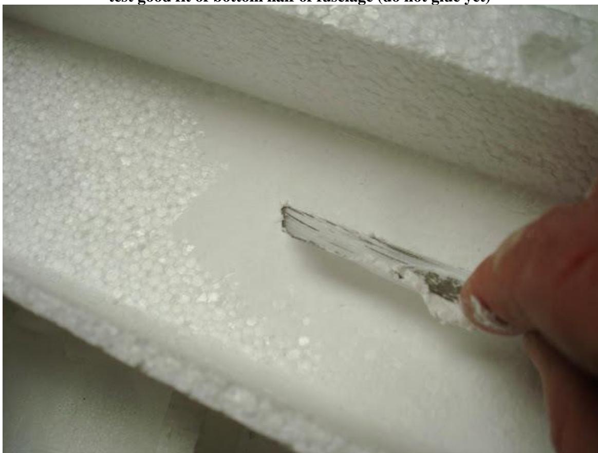
use some easyfiller to make bottom insert smooth before it is glued together
