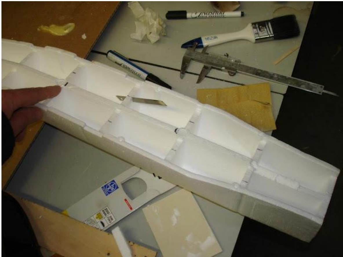
50mm wide battery tunnel has to be created
