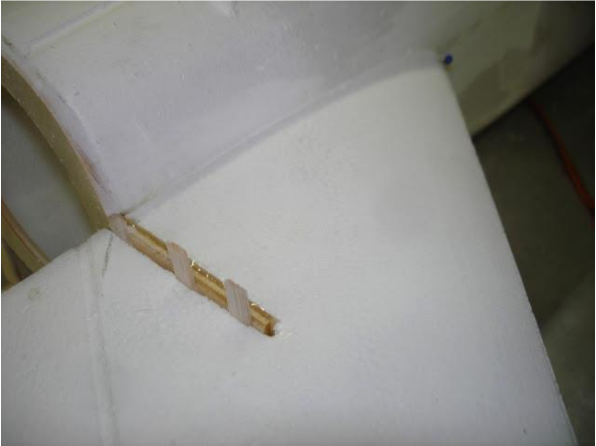
to keep elevator in position: push in small pieces of Balsawood
