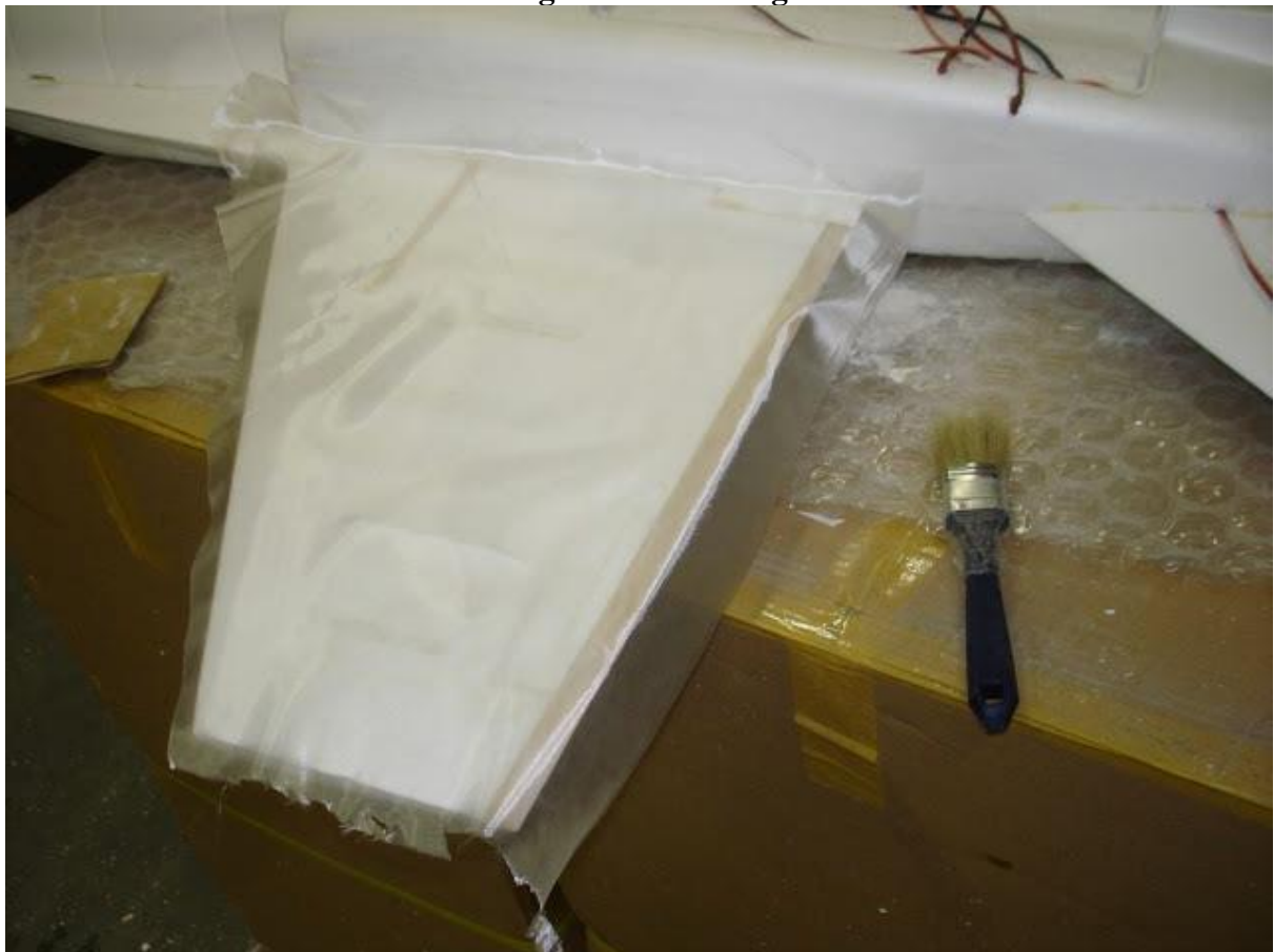
Glassing wing with 25 gram glass tissue and HT-2 Epoxy
