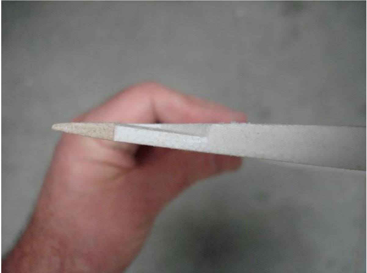
after sanding you have strong balsa trailing edge
