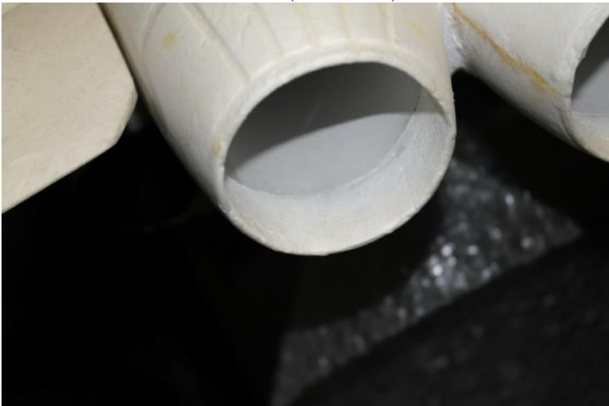
Foam nozzles ends look bigger than they actual are, I did only little sanding on foam nozzle end (inside of foam)
